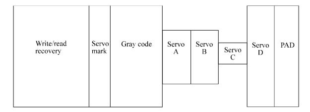
Figure 4.8 Servo frame format
